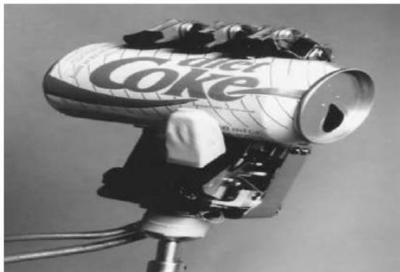
FIGURE 140.10 The Southampton hand prosthesis with four degrees of freedom in a power grip. An optical/acoustic sensor is mounted on the thumb.
