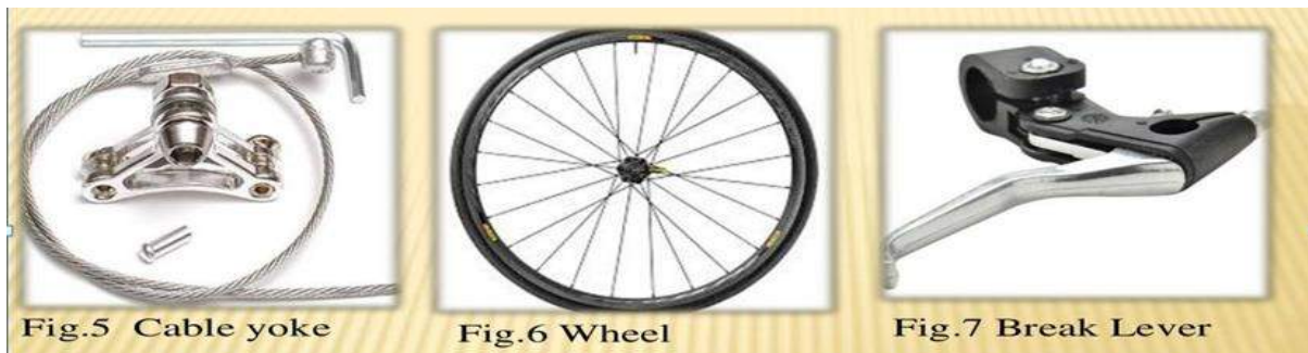
Fig.5 Cable yoke Fig.6 Wheel Fig.7 Break Lever
