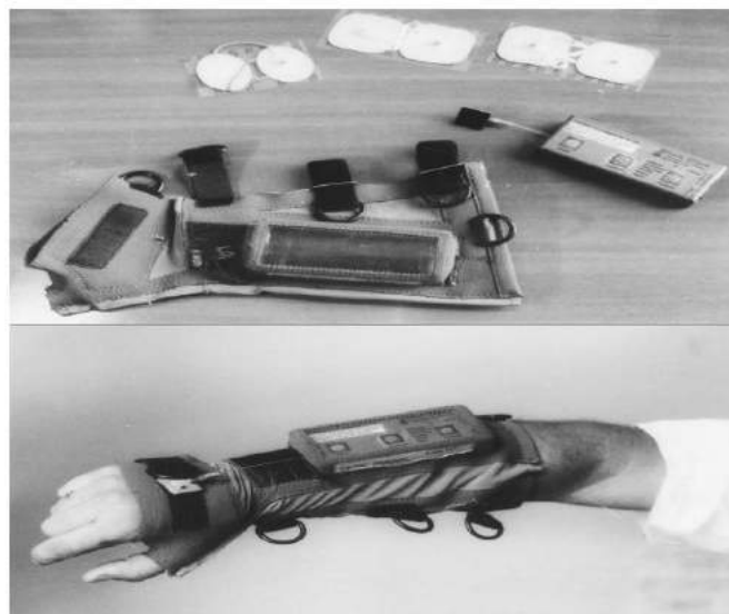
FIGURE 142.1 Bionic glove for restoration of grasping in persons with tetraplegia used for multicentre trials [7,22]. The upper panel shows electrodes, stimulator, and the glove, while the bottom panel shows the glove mounted and ready for use.
